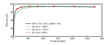
Figure 4: Inverter Efficiency vs. Power Output.
