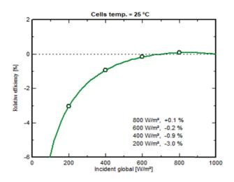
Figure 2: Relative Efficiency With Respect to STC.
