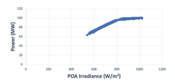
Figure 1: Temperature-Adjusted Power.
