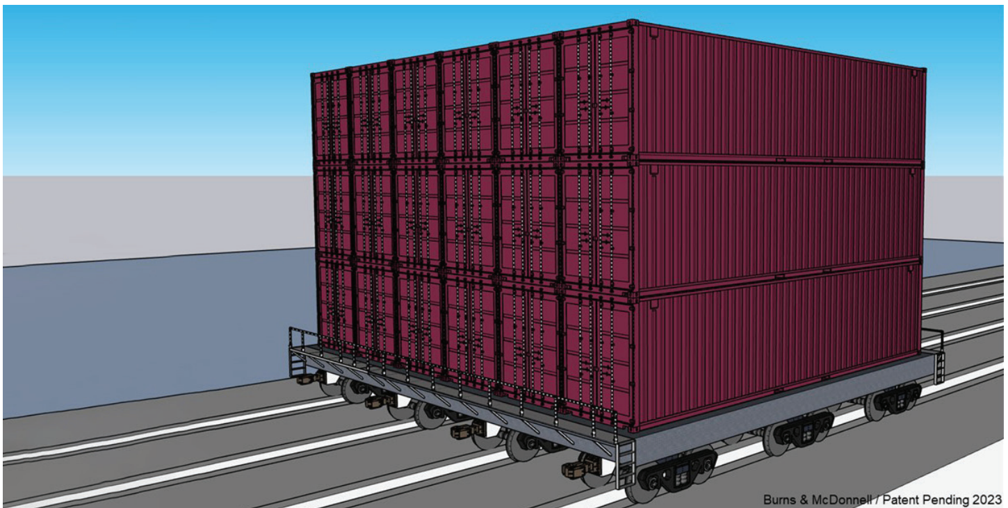
Figure 6: Container block transporter (CBT).
